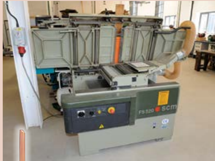
An SCM FS520 planer thicknesser is stood along side the Martin with its 2.3m long tables raised for thickening
