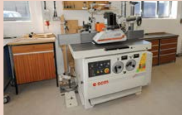
The SCM T150N tilting arbour spindle moulder is also a formidable piece of kit
