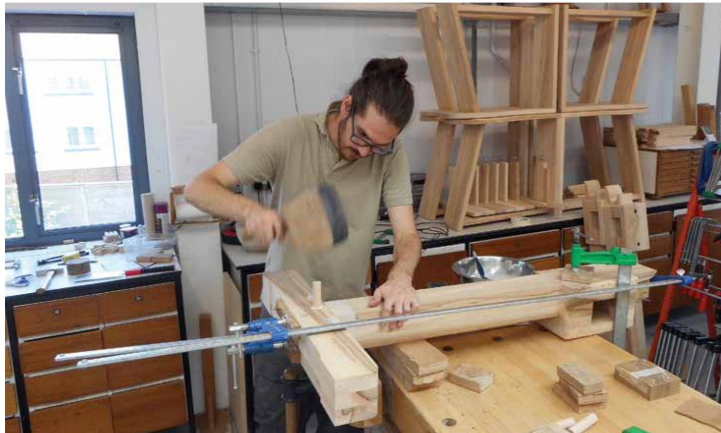
Draw-bored tenons hold the main frame to the feet
