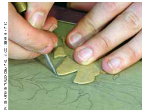
Positioning and marking the individual flowers and elements on the plain background veneer
