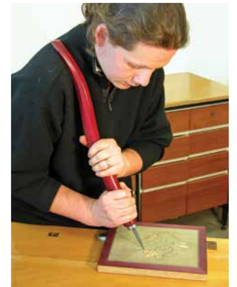
Inlaying the flowers into the background veneer using the shoulder knife
