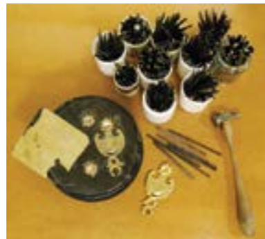
The tools used for chasing. The components are bedded into a block of pitch to hold them while the chasing is done
