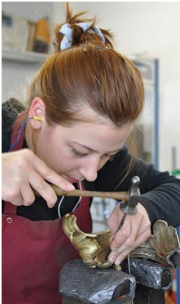
Every square centimetre of the bronze castings has to be finished by hand
