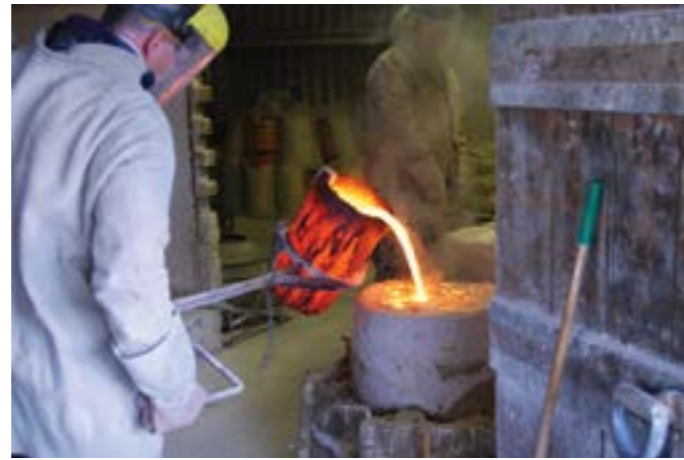
The services of a foundry were used to cast the bronze pieces
