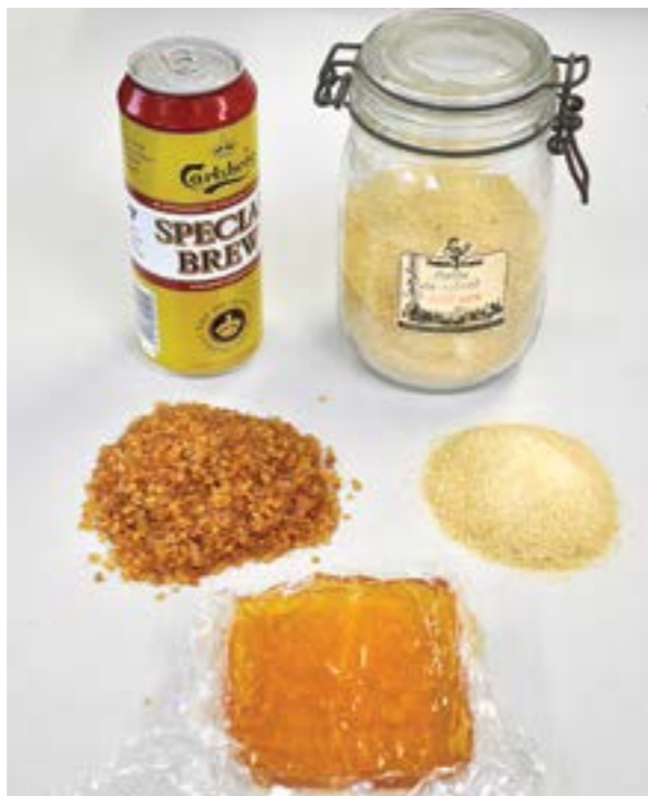
On the left pearl glue from bones; on the right nerve glue in powder form; front, a ready-prepared cake from the fridge ready to be remelted when needed. Note the high-alcohol content beer in the background
