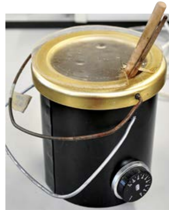
An electric waterless glue pot. The thermo-control means the glue can reliably be kept at optimum temperature
