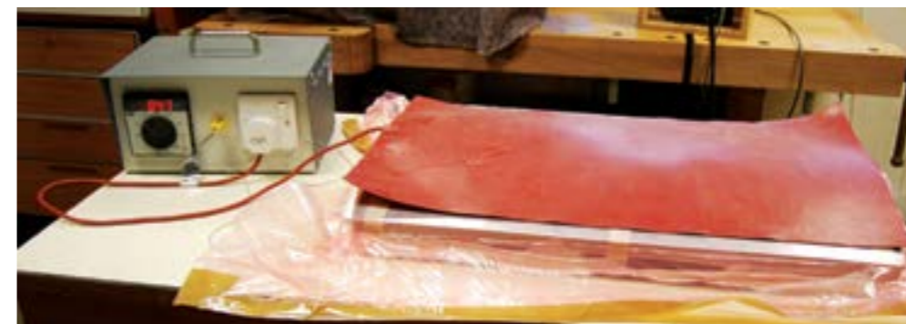
A thermo-controlled heated blanket is the perfect way to keep your woodworking project warm in the course of gluing. It is shown here combined with vacuum clamping, an obvious and simple way of using the heated blanket. The thermo-controlled blanket can also be used in a veneer press
