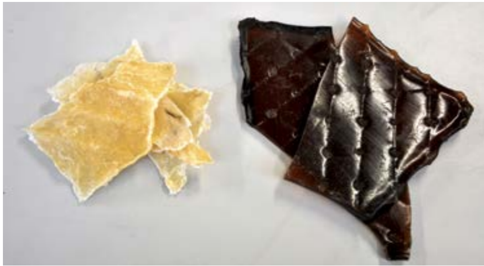
Two very specialised glues in dry form. On the left is one made from sturgeon bladders that need to be cooked in water before using. Sturgeon bladders are reserved for conservation as they are very expensive (£300/kg). On the right is old fashioned colle de givet, sourced from the stock of a retired French cabinetmaker and regarded by French makers as the best
