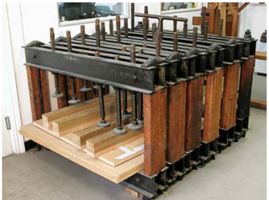
A traditional veneer press that can be used for clamping large surfaces or small items. After years of using vacuum clamping, I find I am more and more returning to traditional clamping because I can obtain a higher degree of pressure. Pressure with vacuum clamping cannot exceed atmospheric pressure while traditional clamping can easily go 3-4 times higher
