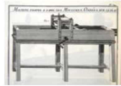
The design of a ripple machine published in André-Jacques Roubo, L'Art du Menuisier Ebéniste , c.1772
