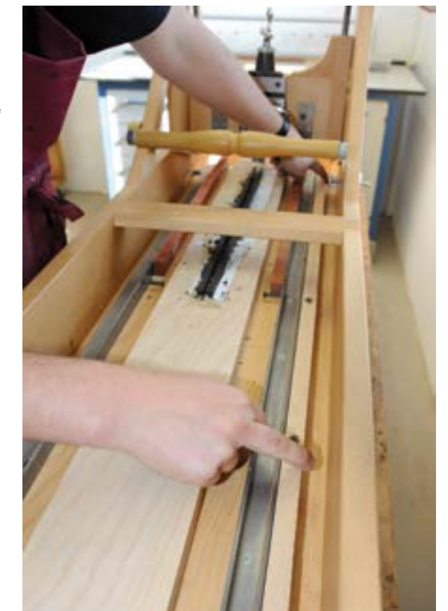
Beech was used to make the guide track that determines the sideways movement of the sliding table
