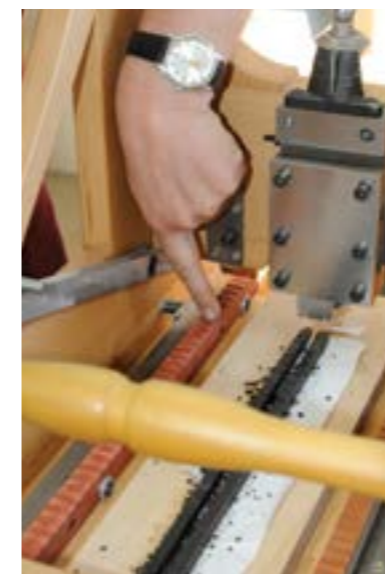
Pink ivory was used as the guide track to activate the rise and fall of the cutter block
