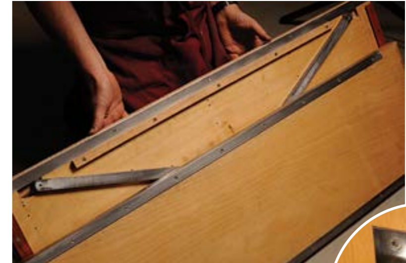
A 'shop-built scissor action guide was used to distribute pressure evenly across the bottom table as it passed through the machine
