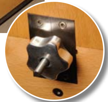
Pressure across the table is maintained and adjusted from a single knob on the side of the box frame
