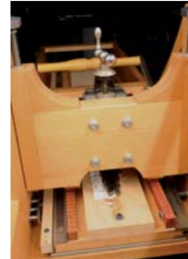
A rigid beech frame was used to build the machine to withstand the forces of the sprung mechanism
